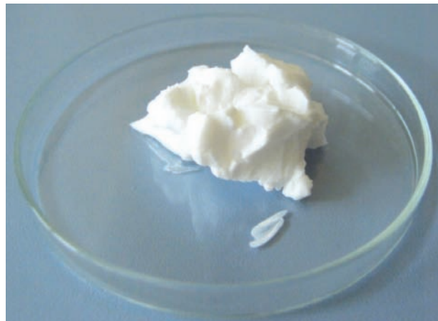
Figure 1—A sample of chemically precipitated calcium aluminate sulphate –ettringite
